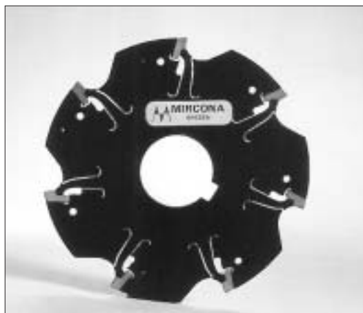
THG 2000 is a suitable material for various types of milling cutter bodies.
