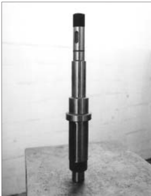
A transmission part manufactured from THG 2000, hardened to 45 HRC.
