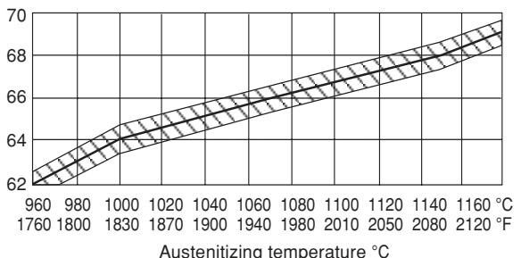
*Hardness for different austenitizing temperatures after tempering 3 times for one hour at 560°C ( $\pm 1$  HRC).*
